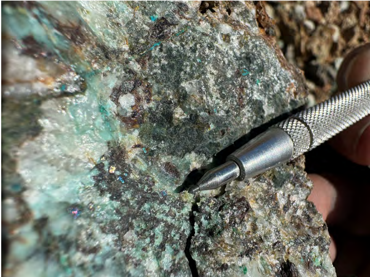
Figure 4: Rock sample with Chalcopyrite and Bornite grading 1.36% copper associated with the leach cap.
